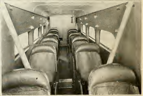
Passengers' cabin of the latest Stinson Model U Trimotor showing the improved seating arrangement for ten passengers
